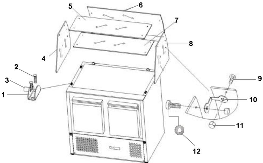
1. First, attach the glass supports (1) (2 on the left, 2 on the right and 2 at the rear) on the housing of the saladette. Use the supplied screws (2).
