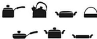
Due to a specific way the induction plate operates, only cookware/containers with a bottom subject to magnetization are suitable.
